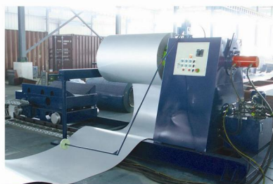
5T/ (5+1)T x 1250mm Hydraulic Uncoiler with Coil Car
