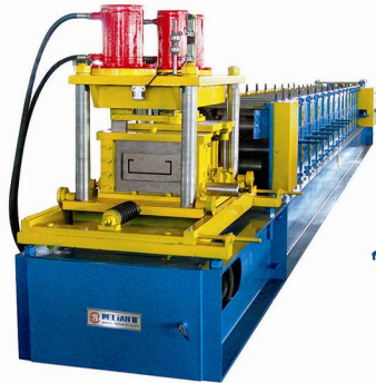
C Purlin with Post-Punching & Post-Cutting
