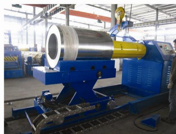
10T x 1250mm Hydraulic Uncoiler with Coil Car
