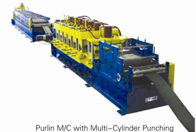
Purlin M/C with Multi-Cylinder Punching (Servo System / Auto Control)
