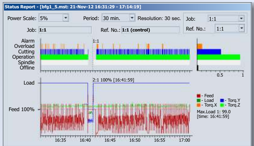
Sample report: Machine utilization over a 30 minute production period
