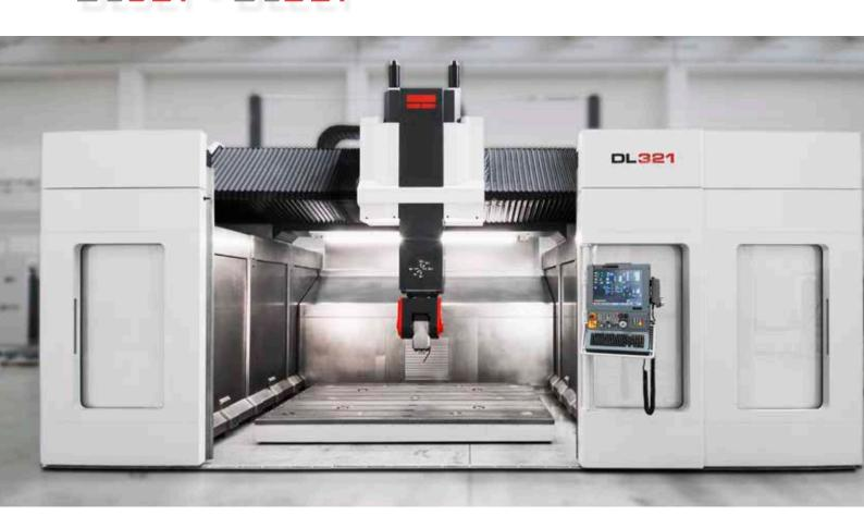
On the DL321 direct linear motors replace the re-circulating ball screws on the X & Y axis, reaching a speed rate up to 60m/min.
