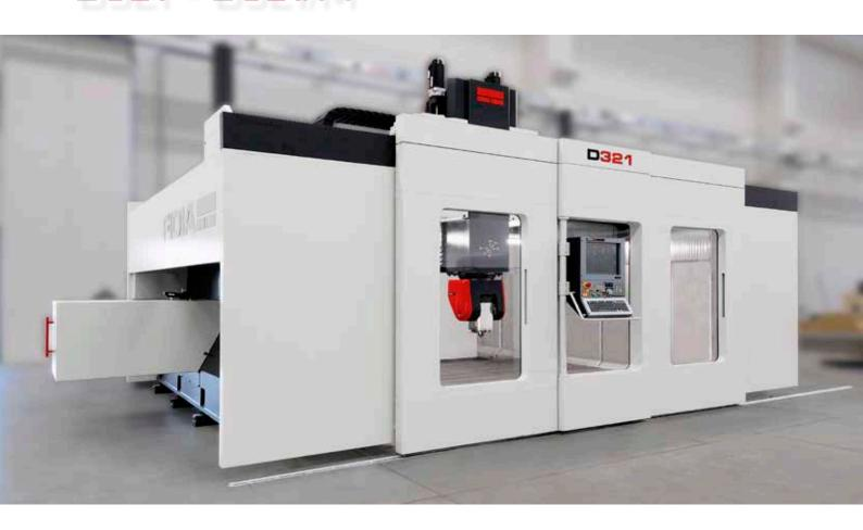
What makes the D321/M different from the standard version is that it features a cast iron base that integrates the work-piece table, creating a monolithic structure.
