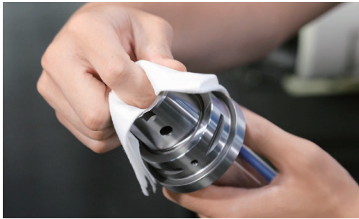
Wipe down the taper of spindle master bar.
