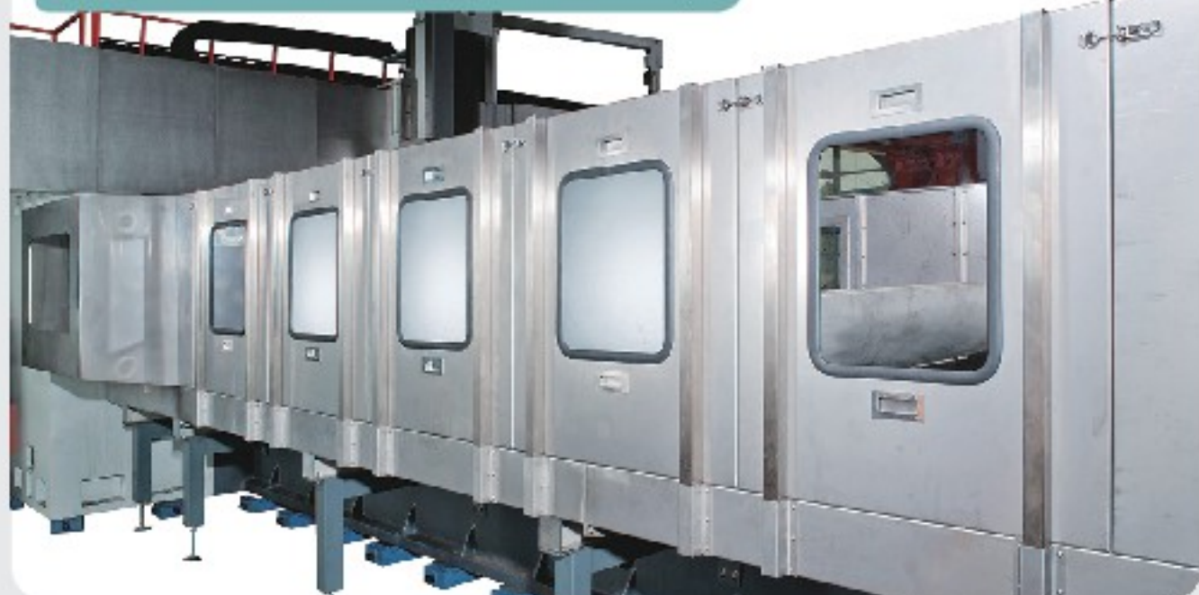
可拆卸式不銹鋼視窗門 Detachable stainless steel window door (選配 opt.)
