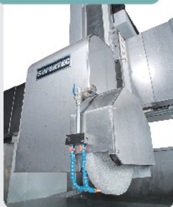
動壓主軸砂輪頭 Hydrodynamic spindle wheelhead
