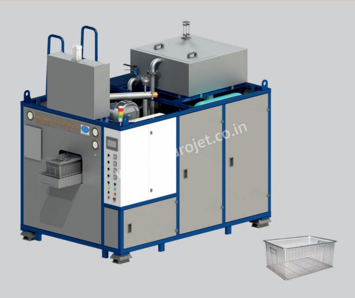
The Multi process cleaning machines are designed for ensuring & achieving excellent cleaning results. All the process such as Spray Washing, High power injection flood washing, Ultrasonic cleaning, Hot Air blowing & Vacuum Drying are carried out in a sequential manner to get desired quality of the component cleaning.
