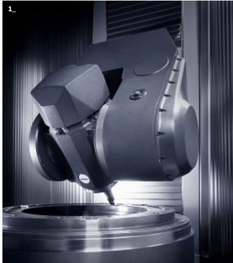
1_ THR 30 MULTIPROCESS: Model equipped with an A-axis THR spindle for machining negative angles ( +45^\circ / -135^\circ ). With a maximum turning diameter of 3000 mm, it allows turning operations at a maximum of 200 rpm on workpieces up to 14t.
