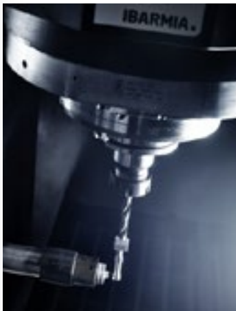
MACHINE PRESETTING DEVICES The program offers the possibility of add a wide range of tool measuring and touch systems integrated in the machine.
