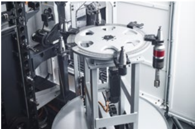
INTEGRATED PICK UPS For the management of long and/ or heavy tools, which offer an ergonomic and simple compact solution to expand the range of available tools.
