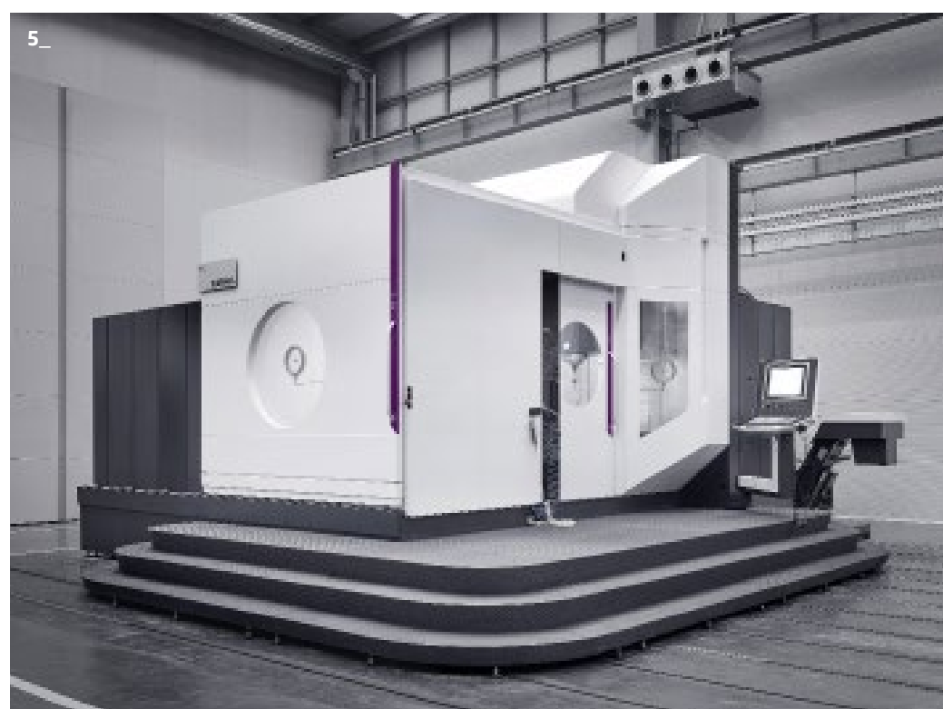
5_ THC 22 EXTREME with the working area completely encapsulated and accessible from the front and lateral sides of the machine. The stepped platform, which is standard for the 12, 16 and 22 models, allows convenient and immediate access to the machine. The T16 and T22 centres offer the option of plastering the machine, while in the case of the T30 and T36 the machine must be plastered without the access platform.
