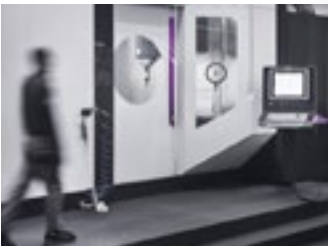
Totally encapsulated working area and safety windows.
