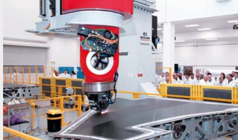
**Mongoose™** is Ingersoll Machine Tool's iconic Fiber Placement module. First released in 2009, **Mongoose™** is aimed at the wide-and-high, complex geometry, composite part manufacturing needs. With its unique bundle of extra-large working volume and extremely compact deposition heads, **Mongoose™** has become the equipment of choice to lay up confined, female molds and complex, male geometries.
