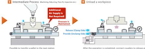
After the operation is completed, connect couplers to release air out. (Provide air pressure to unclamp port to unload a workpiece.)
