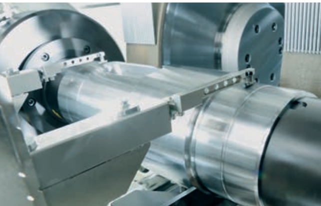
In-process gauging for maximally precise manufacturing
