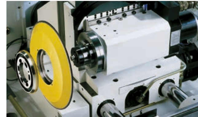
Fast changeover of the wheel with the 3-point mounting system
