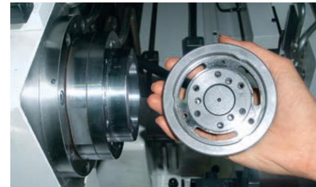
Fast changeover of the wheel with the 3-point mounting system
