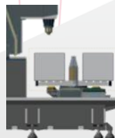
Replacing the fixed table with a 2-axis divider plate
