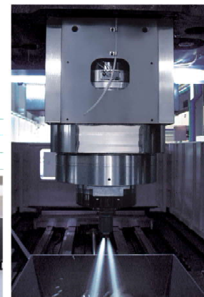
KMC HIS SERIES / Coolant Through Spindle System 13 | 14
