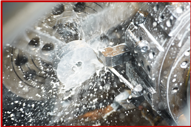
Conventional flood cooling with cutting fluid
