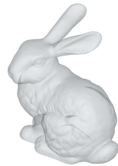
Result of Glue operation – the two parts have been unioned together with no sliver geometry.
