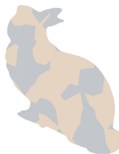
Result of Boolean intersection (grey) plus material added by glue operation (gold)
