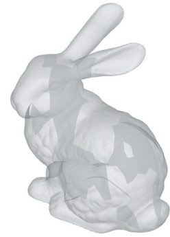
Result of Boolean union – thin slivers of internal geometry remain
