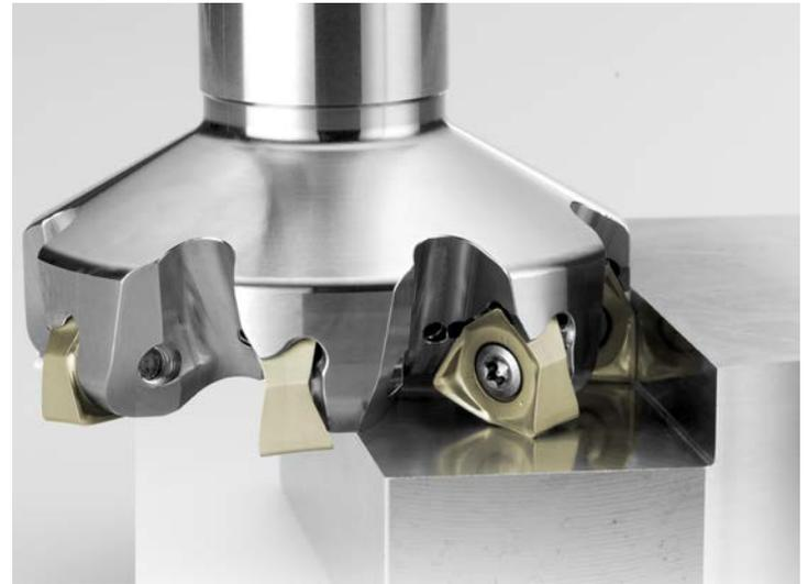
Furthermore, a high maximum depth of cut of up to 8.2mm enables efficient shoulder milling capabilities. In order to meet component surface finish expectations, the bottom of all inserts feature a large radius geometry that acts like a traditional wiper.
