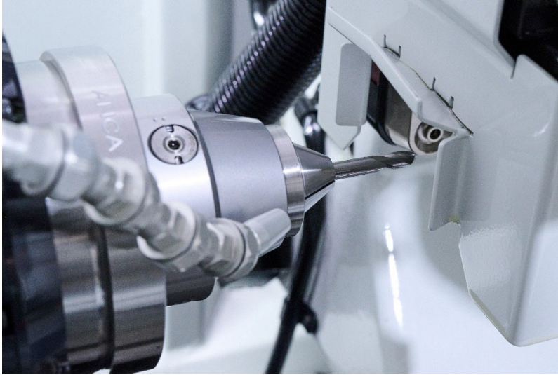
LaserULTRA measuring on FX7 ULTRA
