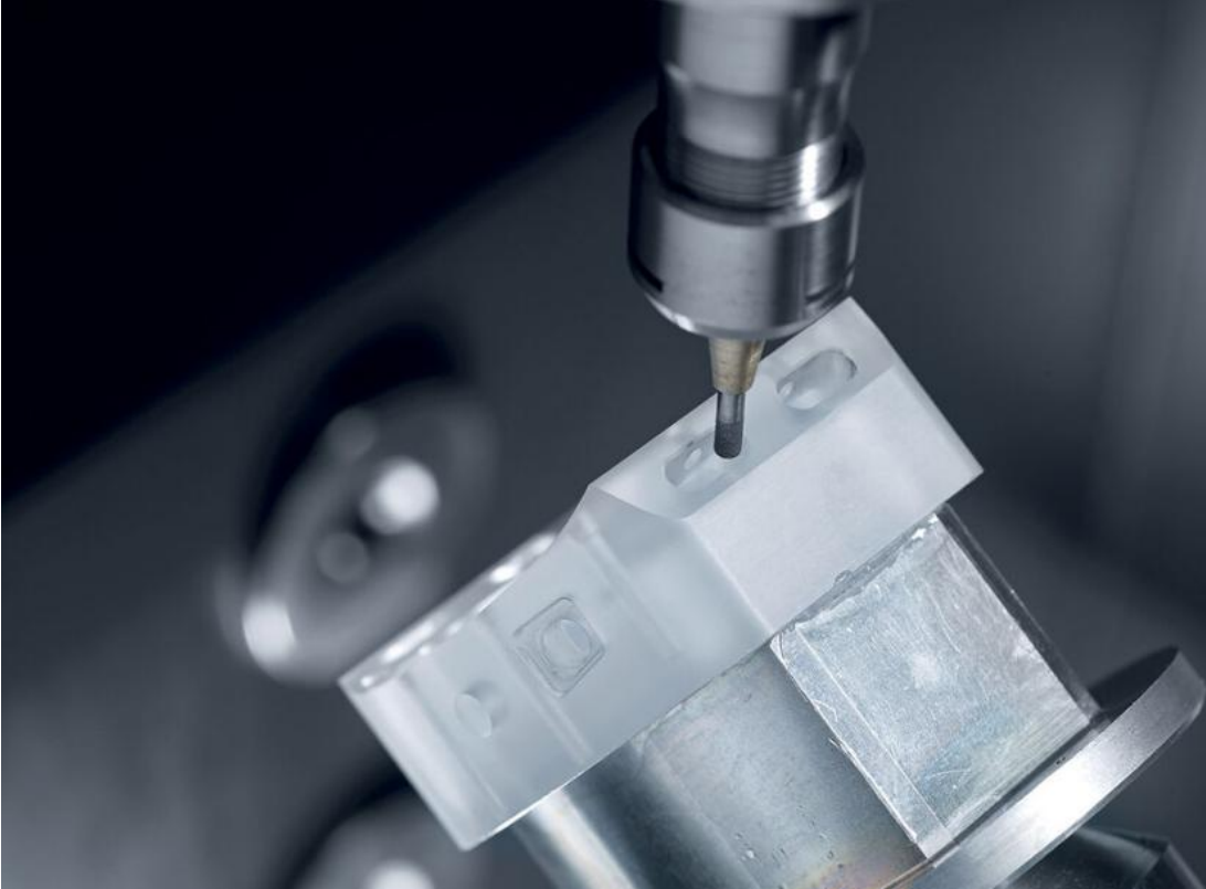
The ULTRASONIC 20 linear 3. Generation revolutionizes ultrasonic-supported milling and (optional) grinding of advanced materials, such as a watch case made of glass here.
