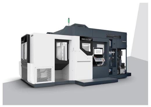
Equipped with two spindles, the DMC 55 H Twin offers double productivity and maximum flexibility on a compact footprint.
