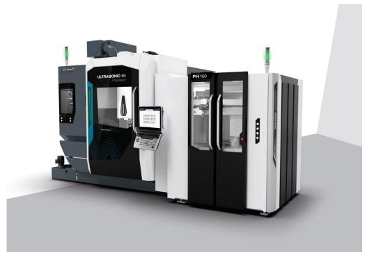
The 5-axis precision ULTRASONIC machining of hard, brittle materials such as silicon carbide or Zerodur is a game changer in the semiconductor industry. Flexible automation solutions optimize the utilization of the ULTRASONIC 60 Precision.
