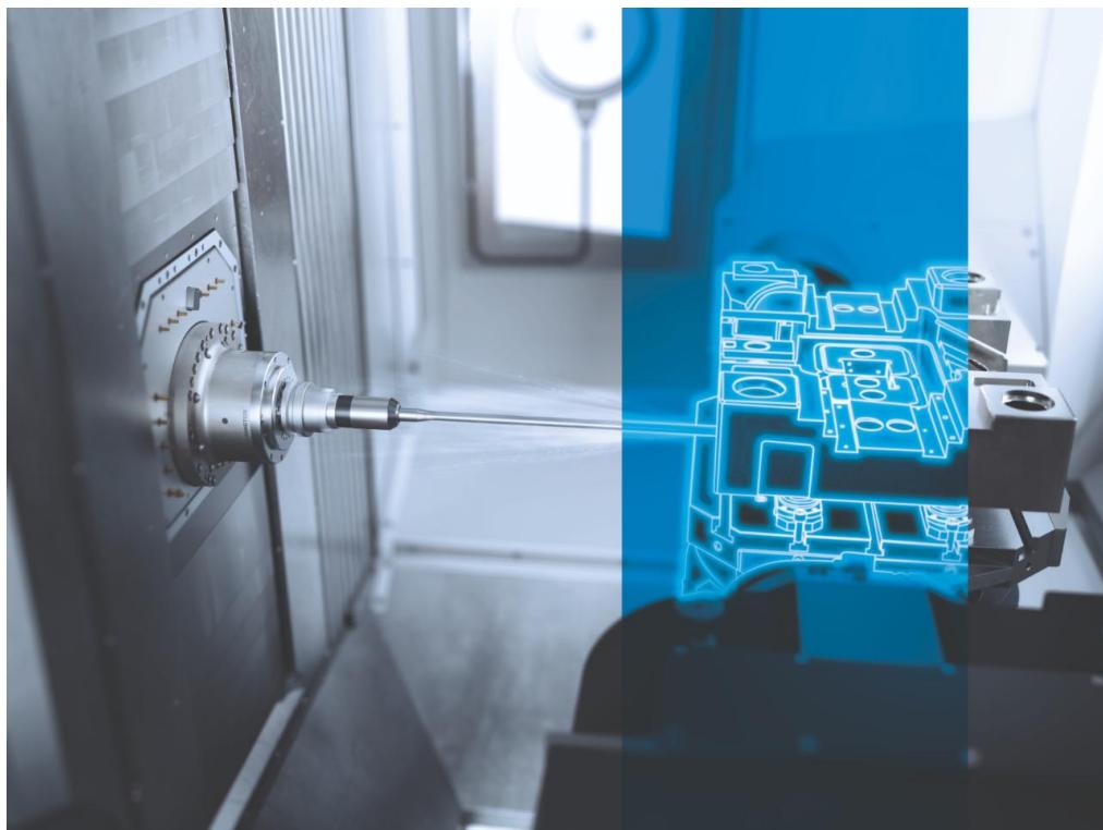
Adaptive Drilling Control (ADC) transforms deep hole drilling, which was previously based on experience, into an actively controlled and monitored drilling process.
