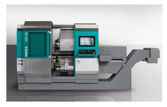
Developed for high productivity and precision, the newly developed CNC automatic lathe INDEX ABC65, successor to the successful INDEX ABC series, uses innovative technologies and proven components from the current INDEX lathe portfolio not only to finish typical machine-turned parts, but also to produce significantly longer and more complex workpieces in large and medium quantities at almost the same footprint.
